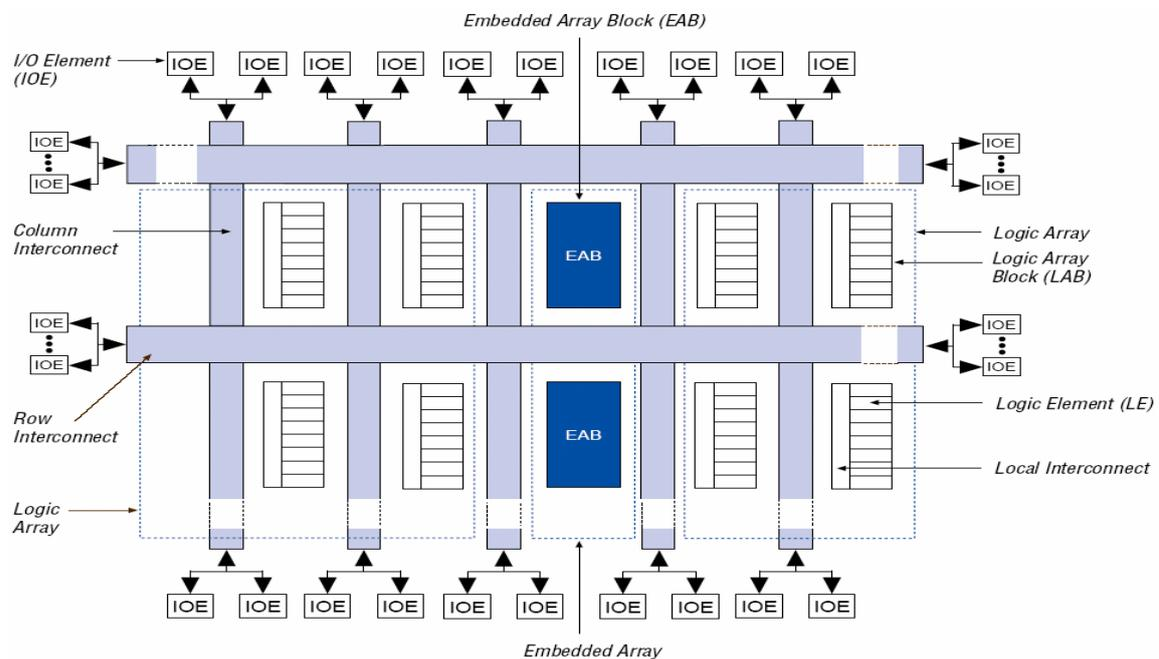
Fig 1. Altera FLEX 10K device block diagram
