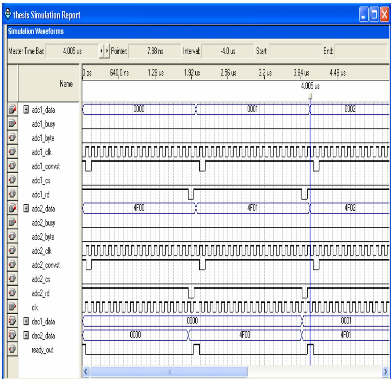
Fig 3. Simulation results of ADC interface
