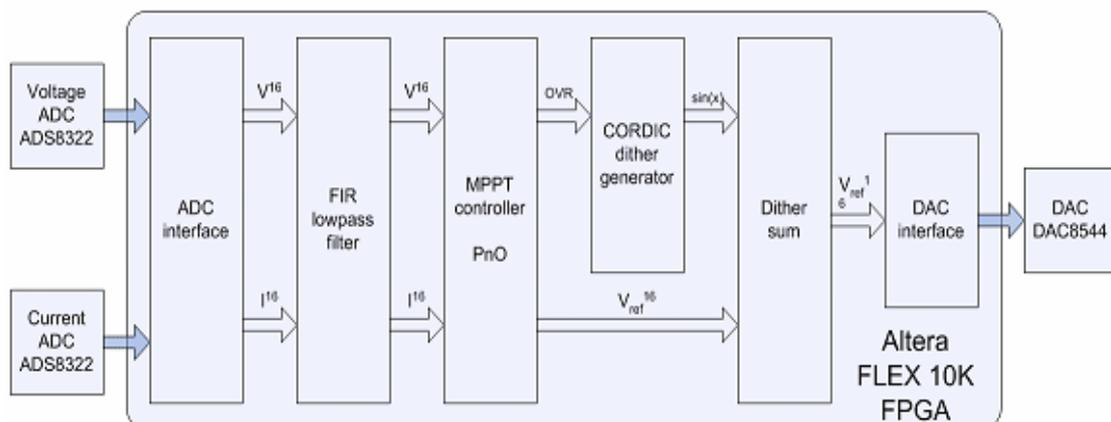
Fig 2. Pipelined system architecture
